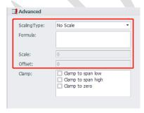
Scaling type specifies how to convert data read from the field device to a number meaningful to users and operators. Specifies how to re-scale input from device into actual Engineering Units. Scaling works with SPAN LOW and SPAN HIGH. Many automation devices supply data a raw form. For example, many 12-bit IO devices supply all values as an integer between 0 and 4096.
