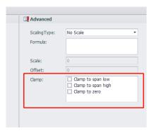
**Clamp to span low**: when the input value is less than the minimum range, the minimum range is displayed.
